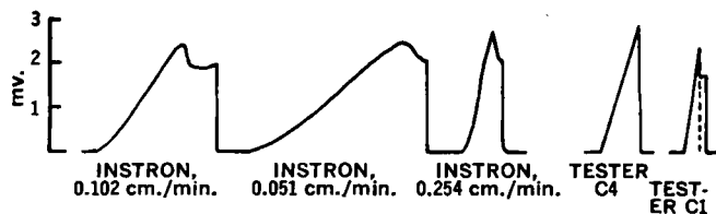
Figure 14—Comparison of the rates of force application for tablets. Tester C4 = a modified Strong-Cobb tester, and Tester C1 = Strong-Cobb tester.
